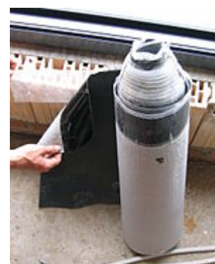
A roll of EPDM flashing with fleece on the back, used for waterproofing roofs
